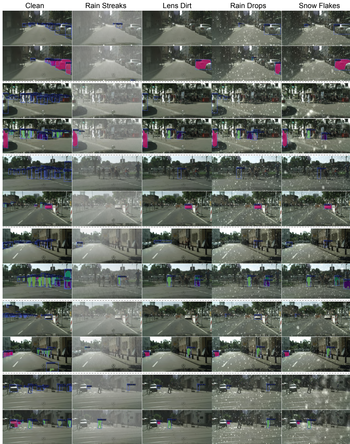
Figure S7. Adversarial Examples of CityScapes dataset. The Object Detection and Instance Segmentation results are shown in the odd and even rows, respectively.
